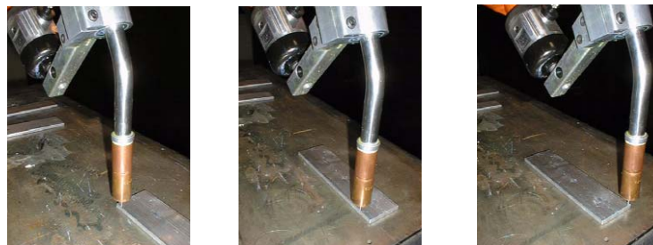
Figure 4-3 Robot arm moves on the same trajectory, however the torch trajectory has changed
